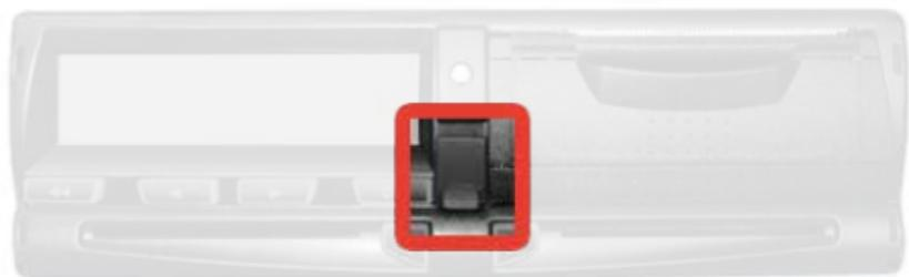
The Actia SmarTach download interface is located on the right hand side next to the display under a flap.
