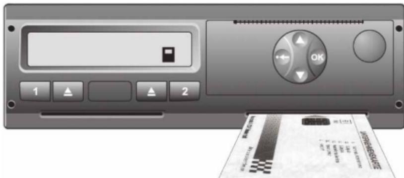
2. Plug the downloadkey in the appropriate port of the tachograph (see page 6-08). The „INIT LED“ will flash for a short while to confirm functionality.
