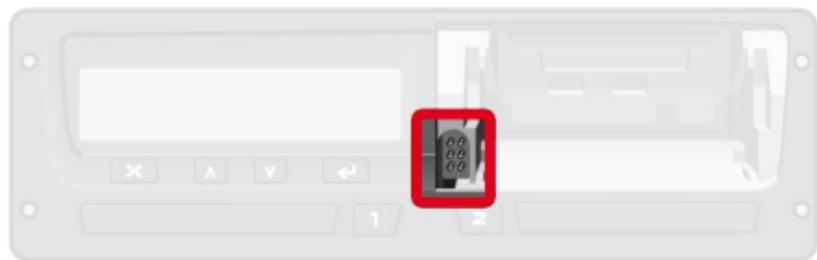
To download data from Stoneridge SE 5000 find the interface on the left side behind the paper tray. Remove the paper tray to gain access to the interface.
